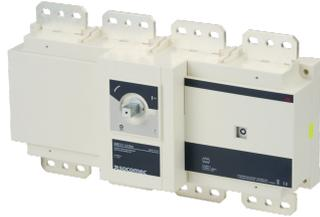
SIRCO AC units are manual or motorised multi-pole load break switches. They make and break under load conditions and provide safety isolation. SIRCO AC devices are designed for extreme applications up to 690 VAC - AC 23.
