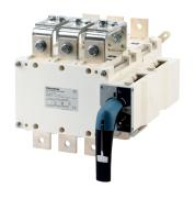
SIRCOVER Bypass provide on-load transfer between two sources for any low voltage power circuit, as well as safety isolation by double breaking per pole. This combination of three interlocked load break switches provides bypass to an UPS or other critical devices, allowing maintenance of a critical equipement while maintaining the supply of the load. There are available in 3 or 4 poles.
