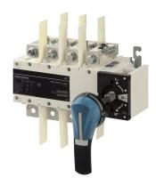
SIRCOVER provide open transition switching (I-0-II), on-load transfer between two sources for any low voltage power circuit, as well as safety isolation with double breaking per pole. In addition to source changeover function, they can as well be used for source inversion (e.g. to change the direction of a motor) or grounding/earthing. They are availlable in 3 or 4 poles.
