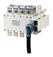
SIRCOVER Bypass provide on-load transfer between two sources for any low voltage power circuit, as well as safety isolation by double breaking per pole. This combination of three interlocked load break switches provides bypass to an UPS or other critical devices, allowing maintenance of a critical equipement while maintaining the supply of the load. There are available in 3 or 4 poles.
