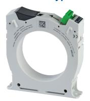
Residual core transformers, including the active conductors, establish the differential sum of the vector currents to detect leakage currents.
