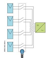
4 MPPT switches, 4 circuits are switched together.
