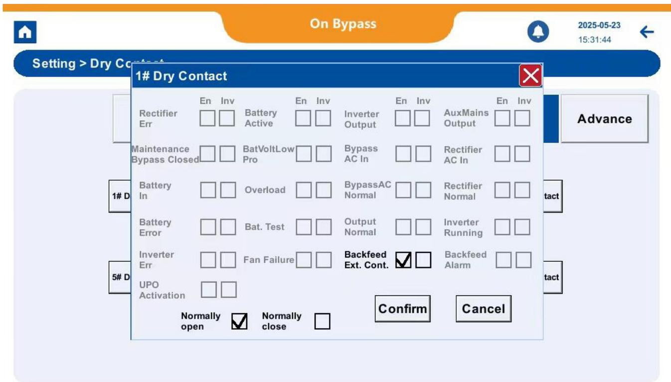
The image above shows a specific configuration setting for dry contact number 1, to activate the backfeed protection function.
