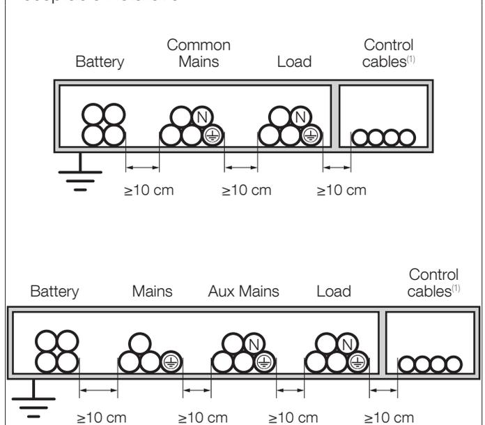
(1) Control cables: connections between the cabinets and each unit, alarm signals, UPO, etc.
