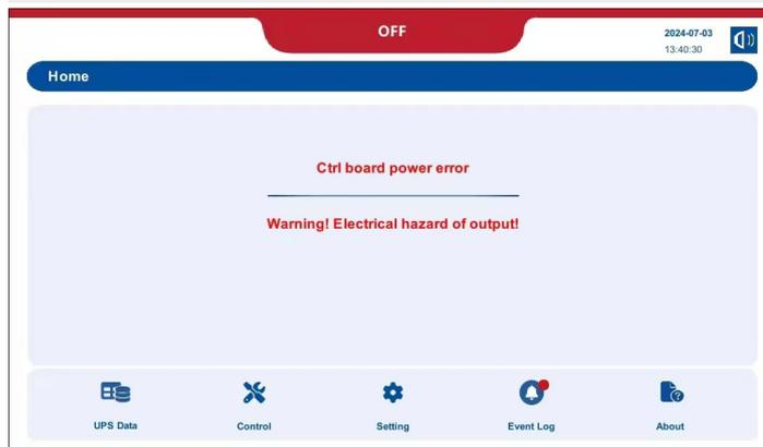
4. When the power supply of the main control board is abnormal, the window pops up automatically.
