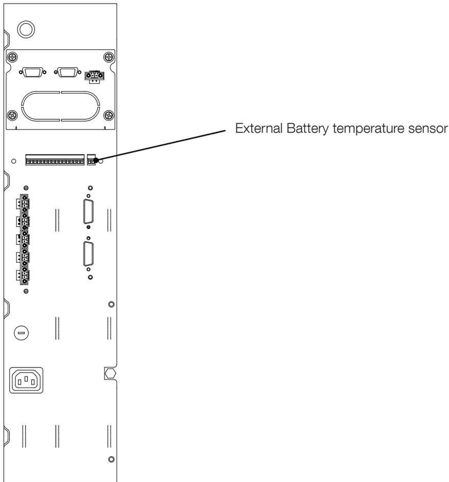
It's possible to configure and enable the battery temperature compensation function on the HMI by service people.
